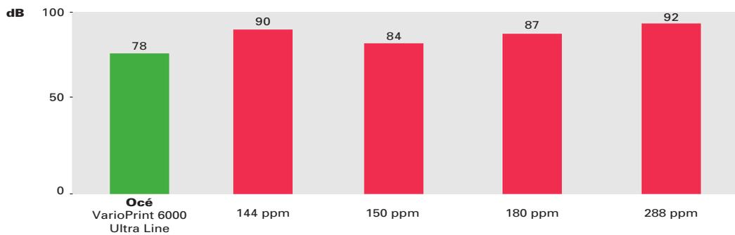
Sound power level (dB) for engines **in standby** for the Océ VarioPrint 6000 Ultra Line and four competition printers
